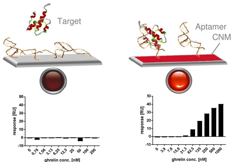
Fig. 1: Top: Principle of a surface-sensitive sensor with immobilised aptamer "receptors". Bottom: Detection of various concentrations of the peptide ghrelin by surface plasmon resonance by an immobilised ghrelin-binding L-aptamer. Left: Target recognition is inhibited by interactions of the receptors with the surface. Right: Using a CNM nanointerposer, aptamers maintain their three-dimensional structure and thus their target binding properties.
