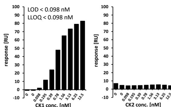
Fig. 2: Specific detection of various concentrations of chemokine 1 (CK1) in UTM by an anti-CK1 L-aptamer immobilised to a CNM on a surface plasmon resonance chip. No binding of chemokine 2 (CK2) to the anti-CK1 L-aptamer. LOD: Limit of detection, LLOQ: Lower limit of quantification.
